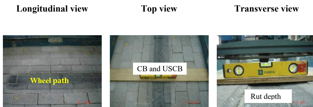
Figure 7.14 Development of rut after several repeated load for USCB and control block (CB)
