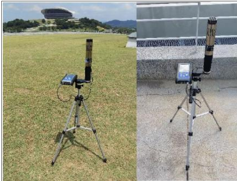
Figure 1: The probe is set up 300 mm above the ground to obtain data
