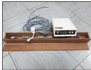
Figure 12: Miniature current meter
