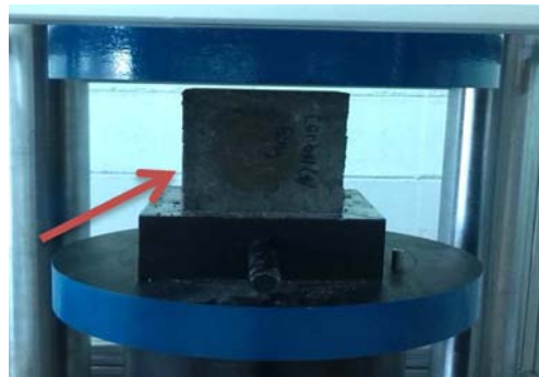
Figure 2: Compression test of concrete
