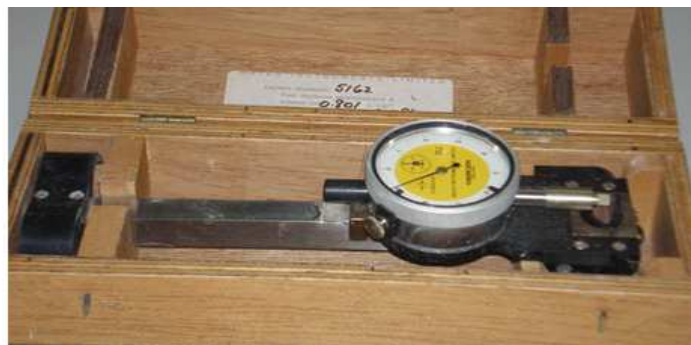
Figure 5: Demec measurement test kit
