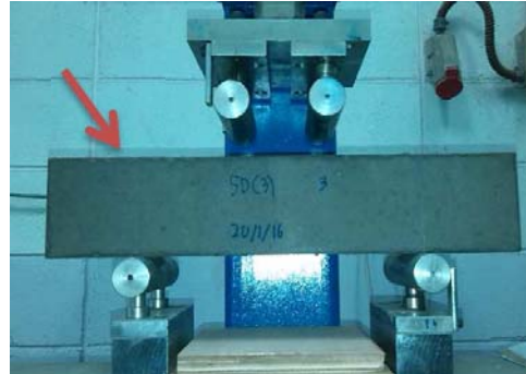
Figure 4: Flexural test of concrete prism
