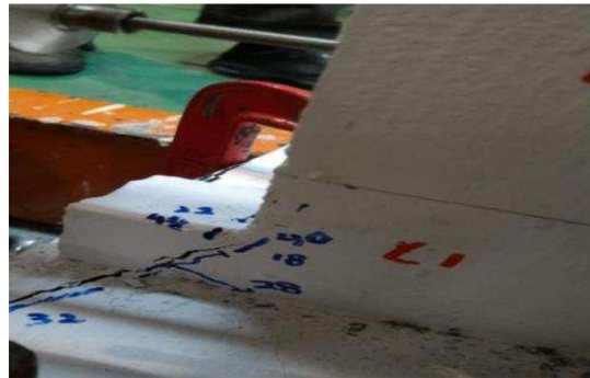
Figure 10: Crack at 44 mm of Displacement and Spalling
