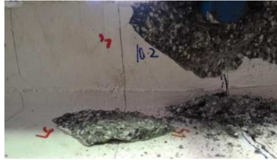
Figure 23: Crushing at 10.2 mm of Displacement
