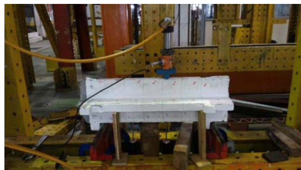
Figure 4: Bending Test Set Up
