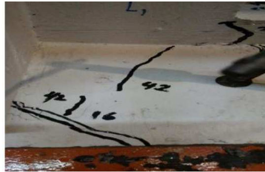
Figure 9: Crack at 42 mm of Displacement
