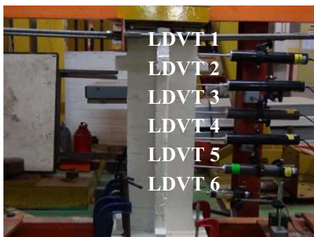
Figure 3: Monotonic Test Set Up
