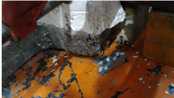
Figure 14: Crushing of Corbel at 32 mm of Displacement
