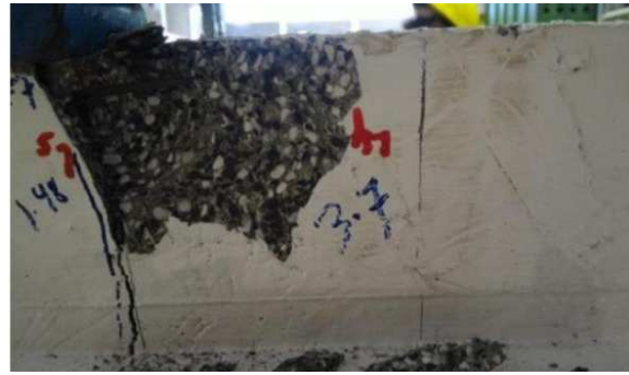
Figure 19: Top Surface Crushing
