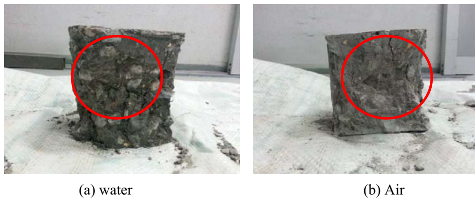
Figure 5: Failure of concrete cube
