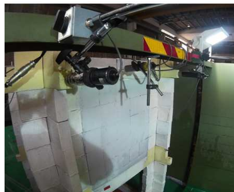
Figure 10: Position of LVDT (50mm) used for all 4 models
