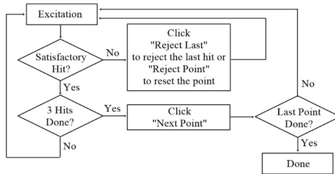
Figure 3: Flowchart showing the Procedure to Roving Hammer Method Modal Test
