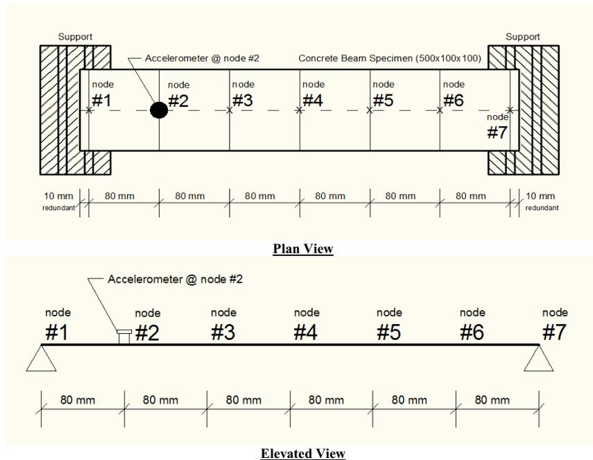
Figure 2: Depiction of Concrete-beam Specimens Setup with Labels during Modal Tests (Not to Scale)
