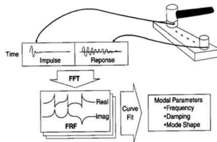
Figure 5: Signal Post-Processing Steps
