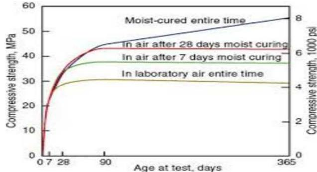
Figure 1: The Influence of Moist Curing on the Strength of Concrete [4]
