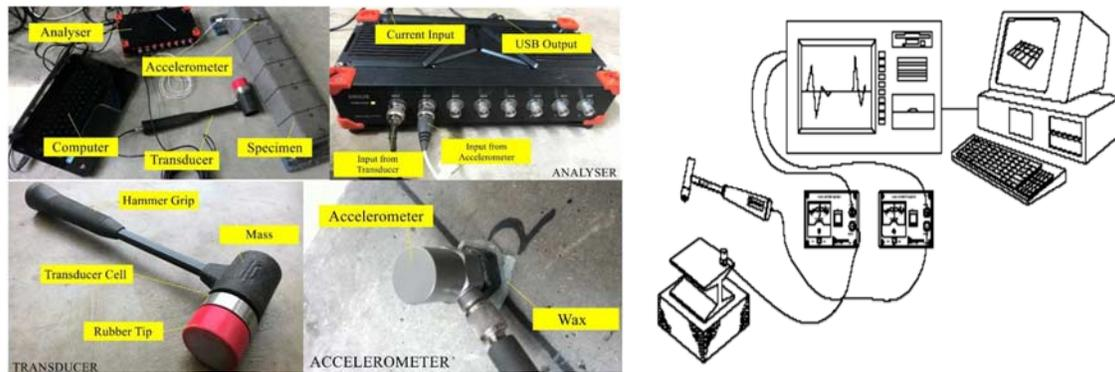
Figure 4: Setup of Modal Hammer Testing
