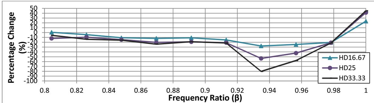
Figure 14: Performance difference compared to structure with TLD at frequency ratio range below resonance for acceleration control
