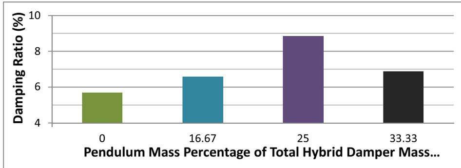
Figure 6: Damping ratio of the structure-damper systems
