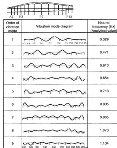
Figure 2: Vibrational modes of the Trans Tokyo Bay Crossing Bridge over multiple frequencies
