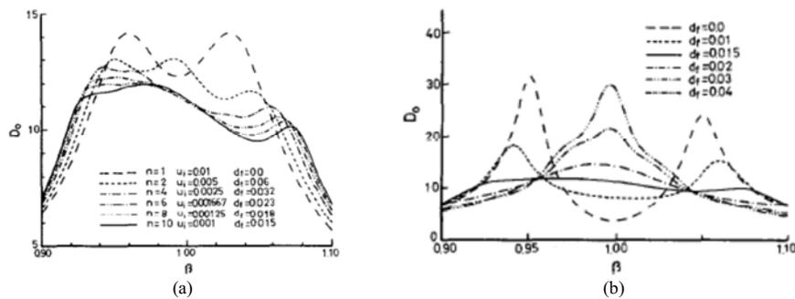
Figure 1: Dynamic response results with (a) varying number of TMD and (b) varying distribution of TMD mass ratio
