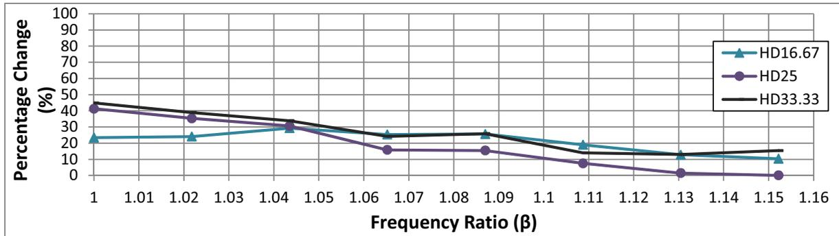
Figure 16: Performance difference compared to structure with TLD at frequency ratio range above resonance for acceleration control
