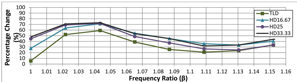
Figure 15: Performance in acceleration response control at frequency ratio range above resonance
