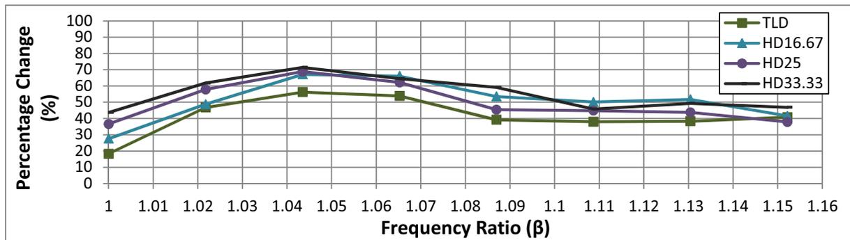
Figure 10: Performance in displacement response control at frequency ratio range above resonance
