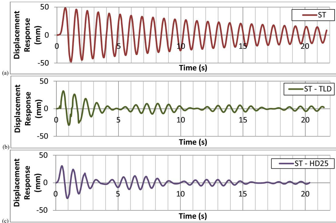
Figure 5: Time history of displacement response of (a) bare structural (b) structure-TLD system (c) structure-Hybrid Damper system with TMD mass portion of 25%.
