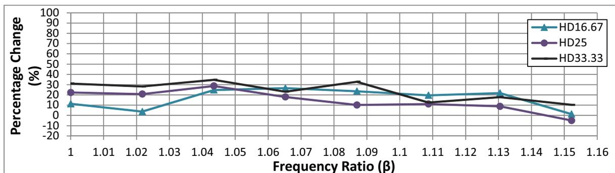
Figure 11: Performance difference compared to structure with TLD at frequency ratio range above resonance for displacement control
