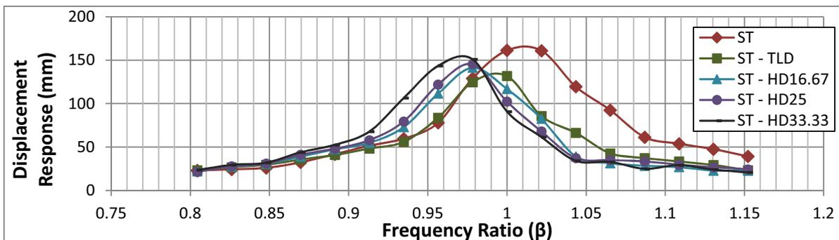
Figure 7: Displacement responses of structural systems against a range of frequency ratio
