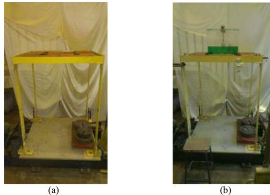
Figure 4: Experimental setup of (a) structure without damper and (b) structure with HD16.67 model installed
