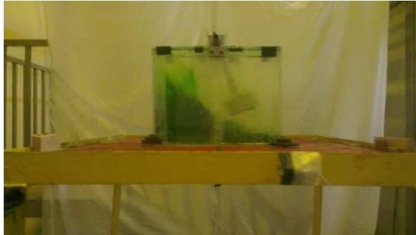
Figure 17: Example of an instant where TMD is completely not submerged in liquid during vibration
