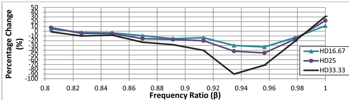
Figure 9: Performance difference compared to structure with TLD at frequency ratio range below resonance for displacement control
