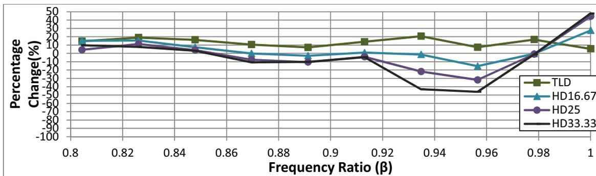
Figure 13: Performance in displacement response control at frequency ratio range below resonance
