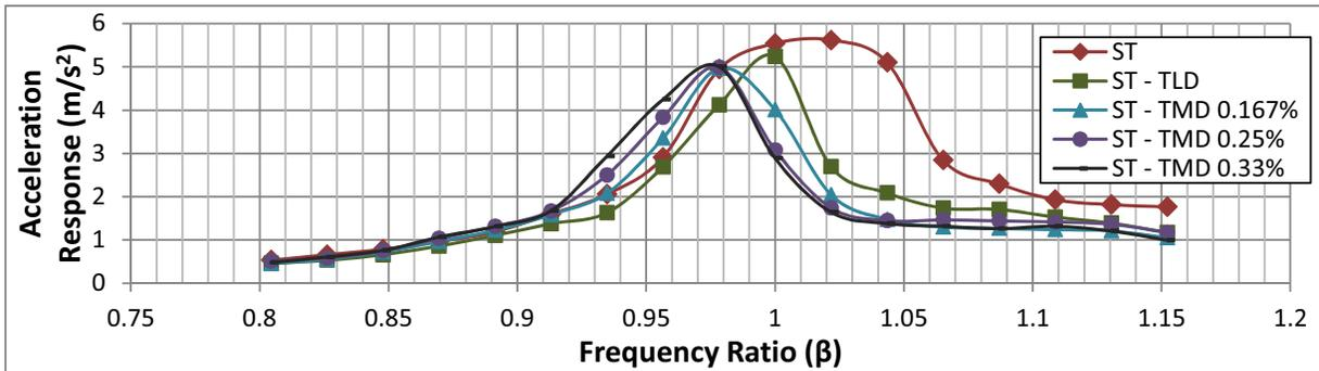
Figure 12: Displacement responses of structural systems against a range of frequency ratio
