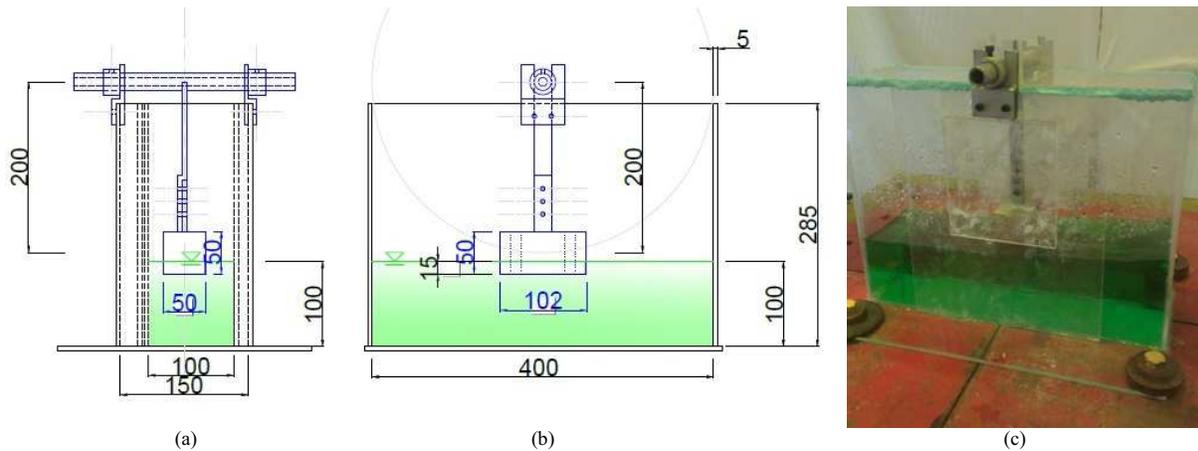
Figure 3: Design specification and dimension of the HD33.33 model in (a) front view, (b) side view and (c) picture of constructed HD16.67 model
