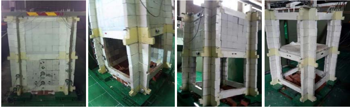
Figure 2: View of models (from the left), full structure, unsymmetrical, symmetrical, and frames.
