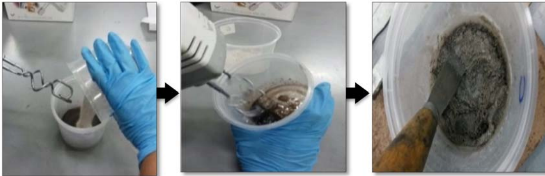
Figure 3: Mixing process of graphene flakes with hardener
