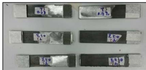
Figure 14: Failure pattern of lap shear test
