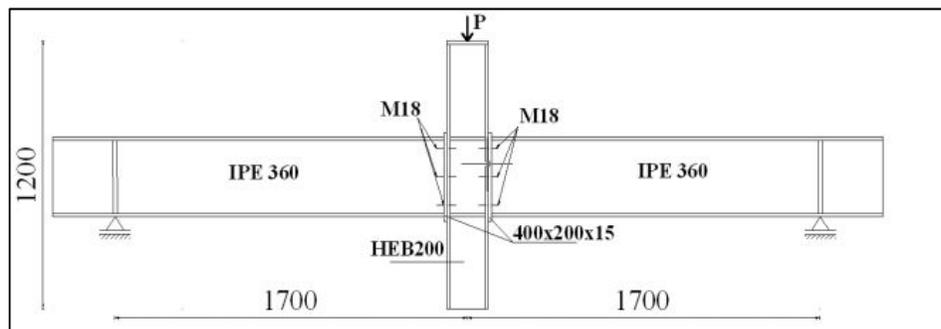
Figure 1: Geometry of test specimen [3]
