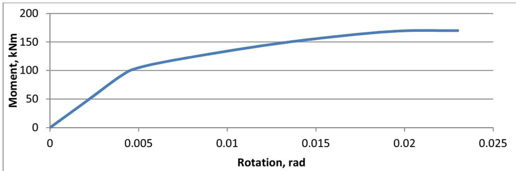
Figure 4: Moment-rotation (M- $\theta$ ) curve of experiment
