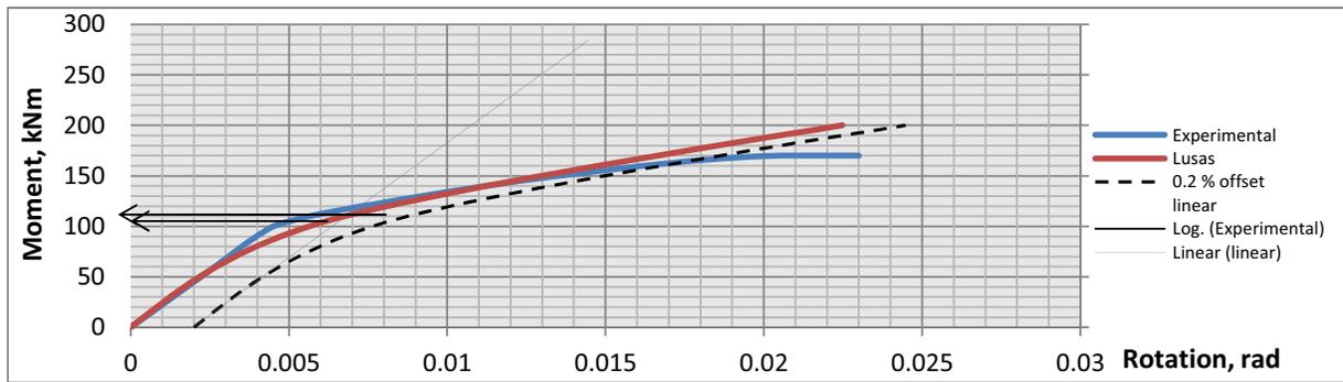
Figure 6: Moment-rotation curve for experimental and finite element model
