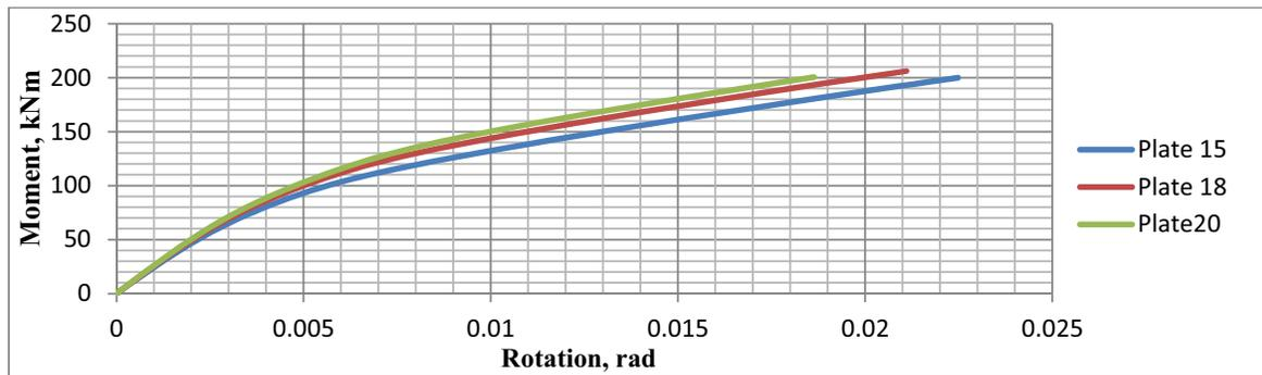
Figure 11: Moment-rotation ( $M-\theta$ ) curve for three thickness of end-plate
