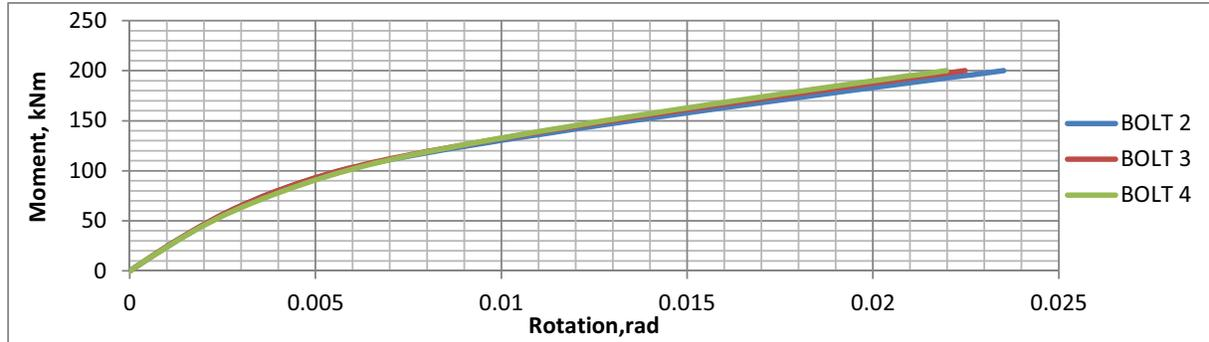
Figure 10: Moment-rotation ( $M-\theta$ ) curve for three number of bolt
