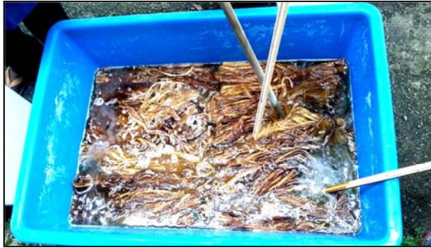
Figure 5: Treatment of kenaf fibers with sodium hydroxide
