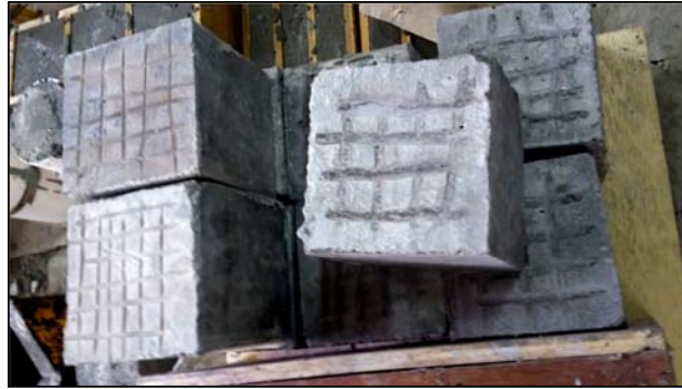
Figure 6: The roughness surface pattern of old normal concrete units
