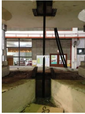
Figure 4: Single-bar tensile test.
