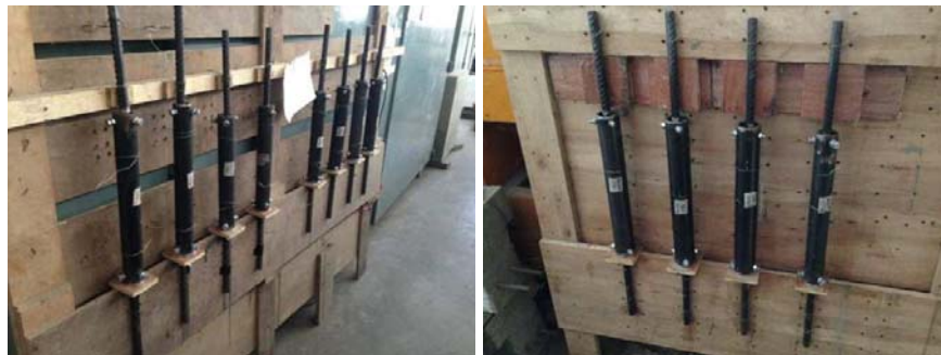
Figure 3: Assembly of the specimens on the plywood frame
