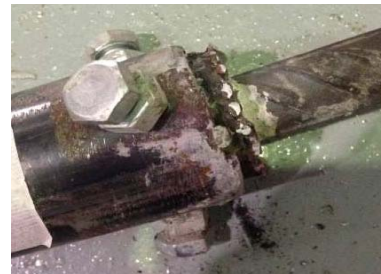
c) Internal sleeve failure
