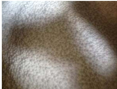
Figure 2: Expanded Polystyrene beads with a size in range of 2.0-3.0 mm.
