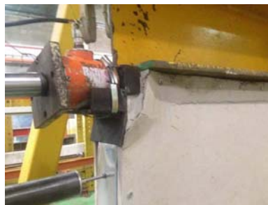
Figure 12: Failure mode of CFS wall frame samples without infill material after tests
