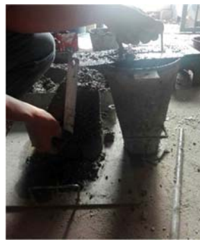
Figure 4: Measure of slump height by using ruler.
