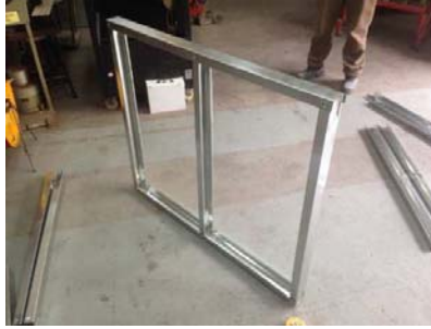
Figure 5: Cold Formed Wall Frame with dimension 980mm x 1114mm.
