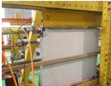
Figure 7: Lateral Load test Setup for CFS wall frame samples.
