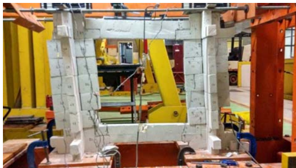
Figure 2: Deformation shape of model at collapse state
