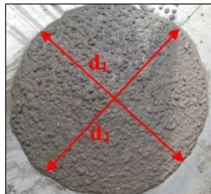
Figure 1. The measurement of slump flow diameter
