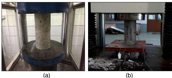
Figure 2. The testing arrangement: (a) cylinder compressive strength test and (b) modulus of elasticity
