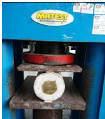
Figure 5. Splitting tensile test
