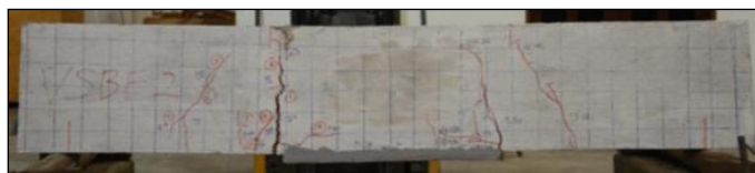
Figure 6. Crack pattern of VSSB
