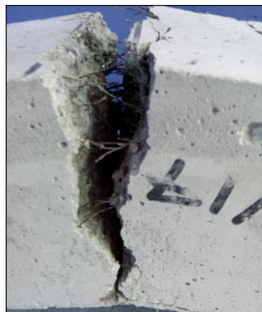
Figure 8. Fibre bridging action in fibre reinforced concrete sample, SFRSCC
