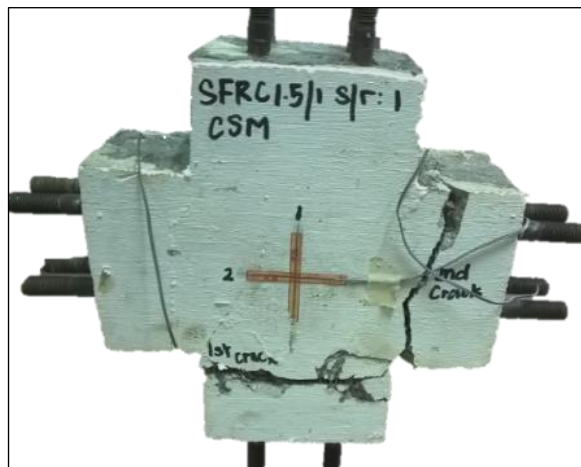
Figure 7. Failure pattern of SFRC with 1.5% steel fibre under stress ratio 1.0
