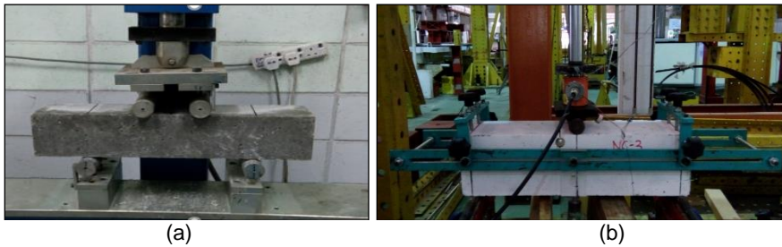
Figure 3. The testing arrangement of (a) flexural strength test and (b) residual flexural tensile strength test
