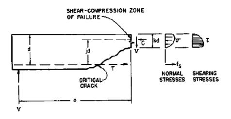
**Figure 2.1** Stress distribution in RC beams (Bresler and Pister)
