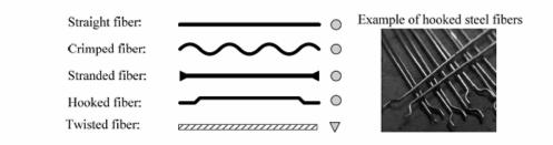
Figure 1.1 Different shape of steel fiber
