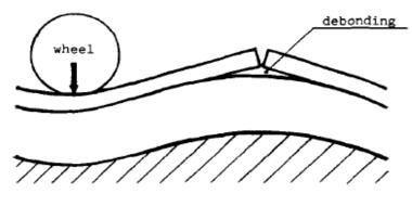
Figure 1.2: Proposed Debonding Mechanism
