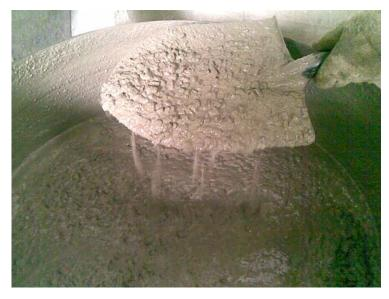
Figure 2.1 : Self compacted concrete
