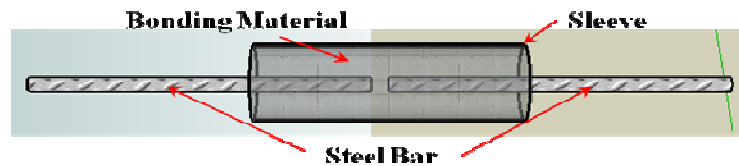
Figure 2.3 Typical splice sleeve connector
