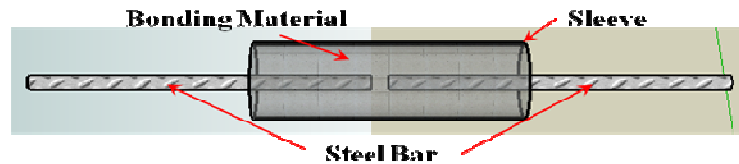
Figure 2.3 Typical splice sleeve connector
