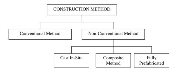
Figure 2.1: Types of construction method
