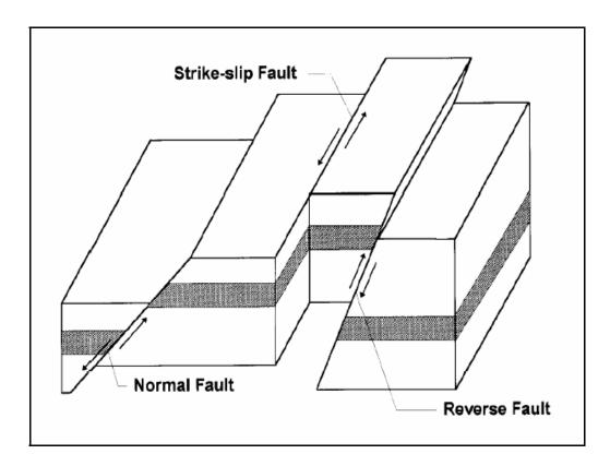
Figure 2.1 Types of faulting
