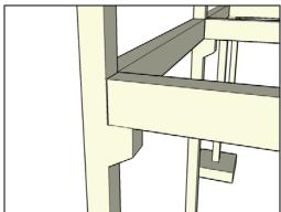
Figure 1.1: The application of simple beam-to-column connections in precast concrete skeletal frame.
