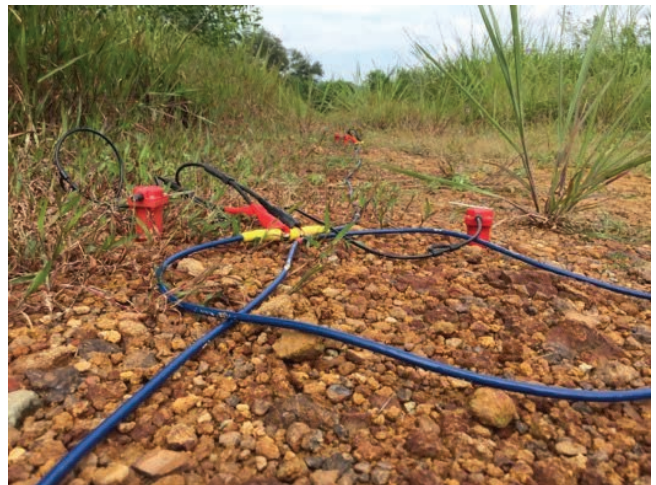
Multichannel Analysis of Surface Waves (MASW)
