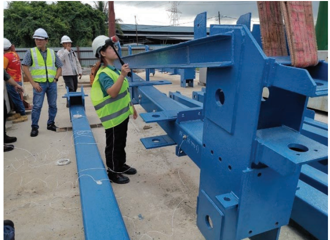
The application of VBDD to assess the integrity of traveller foam for bridge construction.
