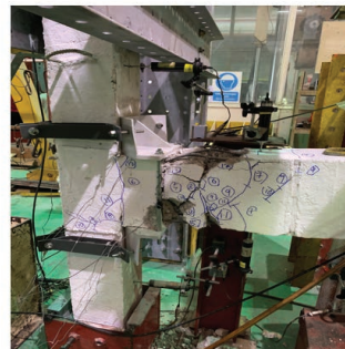
c. Large Pre-tensioned Stiffened Steel Angles
