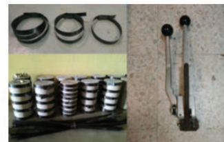
Steel strapping confinement (a) Steel straps; (b) Confined specimens; (c) Tensioner
