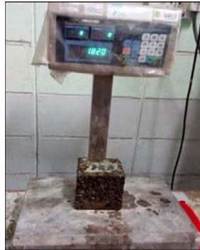
Figure 10: The concrete cube sample is weighed
