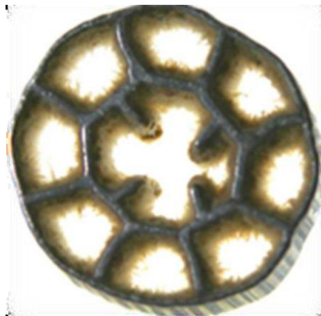
Figure 4: The close up view of Biofilm Carriers that provide enclosed space to support the growth of microorganisms
