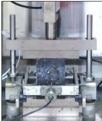
Figure 5: The Resilient Modulus test conducted
