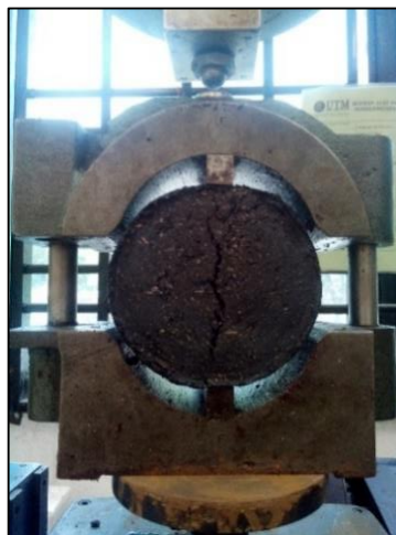
Figure 3: The tensile strength test conducted
