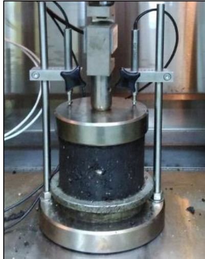
Figure 6: The Dynamic Creep Test conducted
