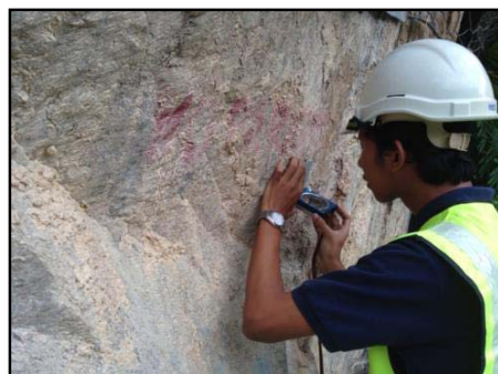
Figure 1: Obtaining Dip Angle and Dip Direction by using Clar Geological Compass
