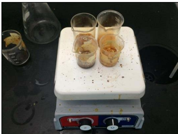
Figure 3: Sample is digested for about 2 hours using hot plate
