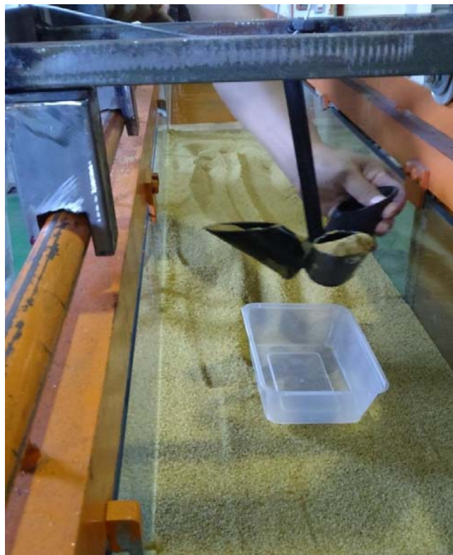
Figure 6: Testing sampler model on the channel
