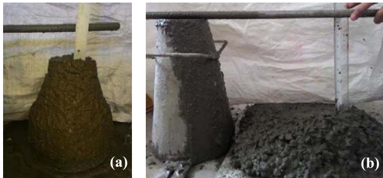
Figure 5: Types of slump for (a) Blended cement concrete and (b) Effective microorganism blended cement concrete
