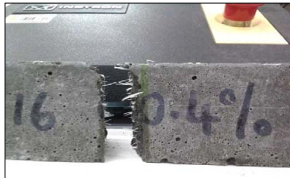
Figure 12: Cross section of samples with fibre after test
