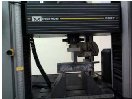
Figure 5: Setup for flexural test
