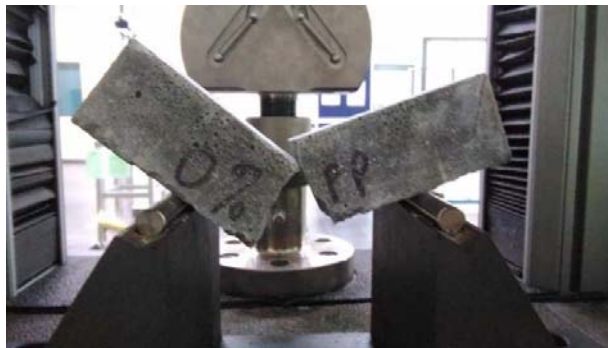
Figure 10: Complete failure of control specimen without the inclusion of fibre
