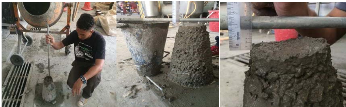
Figure 3: Slump test process
