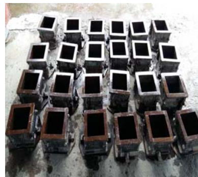
Figure 4: Oiled steel moulds for concrete casting
