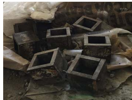
Figure 5: Steel Mould Size 70x70x70mm
