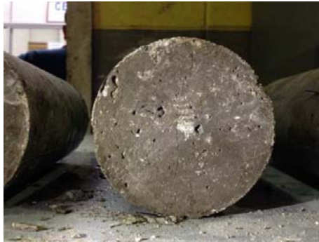
Figure 5: Failure mode for concrete with 3% fibre content due to split tensile
