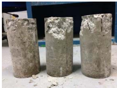
Figure 3: Failure Mode due to Compression.
