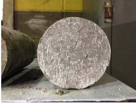
Figure 4: Failure mode for concrete with 1% fibre content due to split tensile
