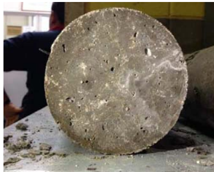
Figure 6: failure mode for concrete with 5% fibre content due to split tensile
