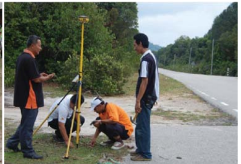
GPS Surveying – To Establish Horizontal Control
