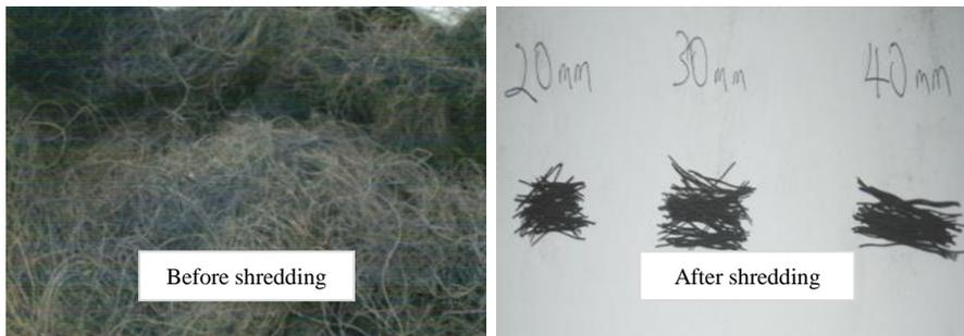
Figure 1: Recycled steel fibre before and after shredding
