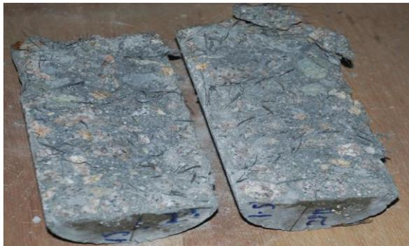
Figure 7: Distribution of steel fibre in broken cylinder.
