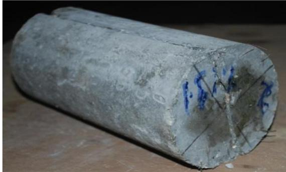
Figure 6: Concrete cylinder after splitting tensile test.
