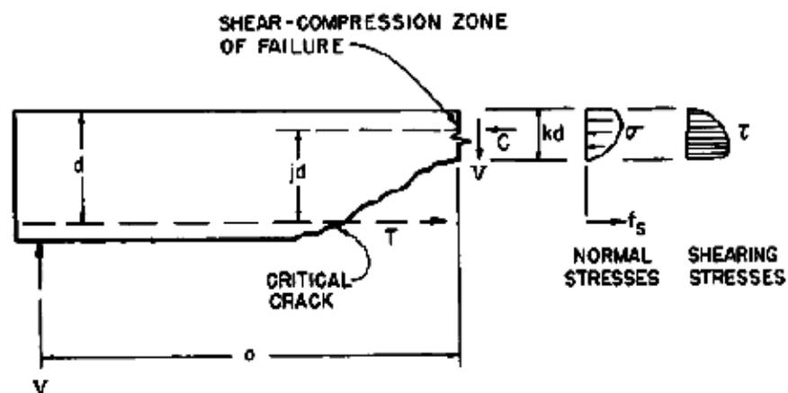
**Figure 2.1** Stress distribution in RC beams (Bresler and Pister)
