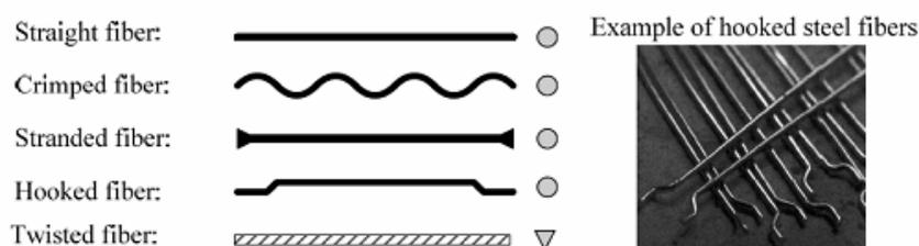
**Figure 1.1** Different shape of steel fiber
