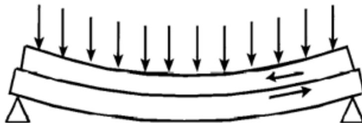
**Figure 1.1: Interface Shear Stress of Composite Member**
