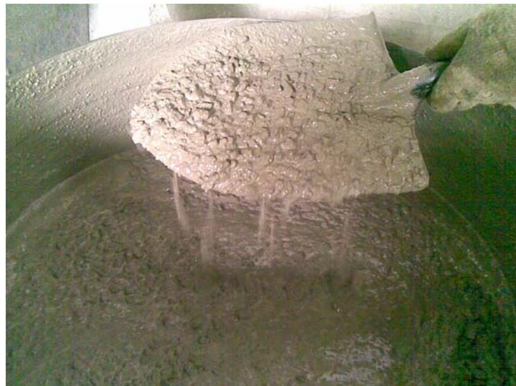
**Figure 2.1** : Self compacted concrete
