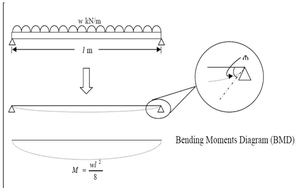
**Figure 2.4:** Simple connections
