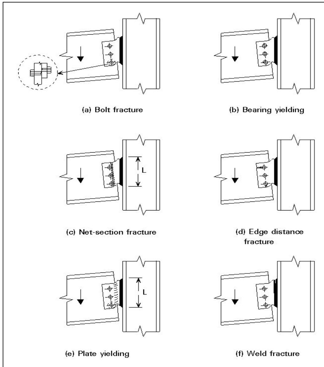
**Figure 2.2:** Illustrates the 6 possible failure modes for a fin plate connection
