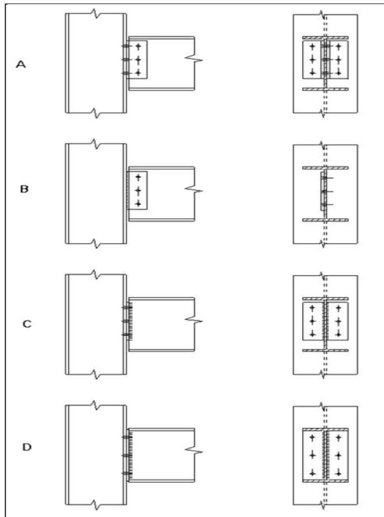
**Figure 2.1:** Beam to column connection, A) fully bolted, B) Finplate C) Endplate, D) Flush Endplate
