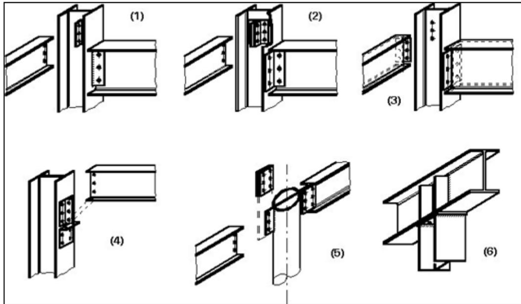
**Figure 2.5:** Simple beam to column connection, 1) fin plates, 2) angle cleats, 3) flexible endplate welded, 4) bolted with angle cleats, 5) tube, 6) stiffness plate
