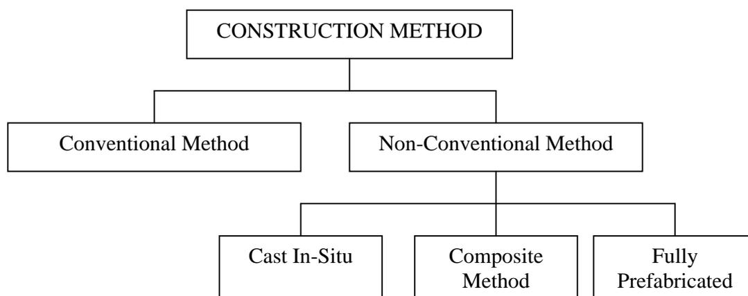
**Figure 2.1:** Types of construction method
