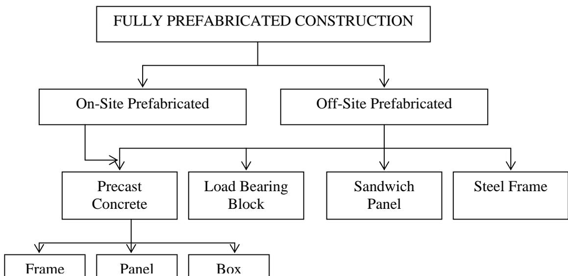
**Figure 2.2:** Classification of fully prefabricated construction method
